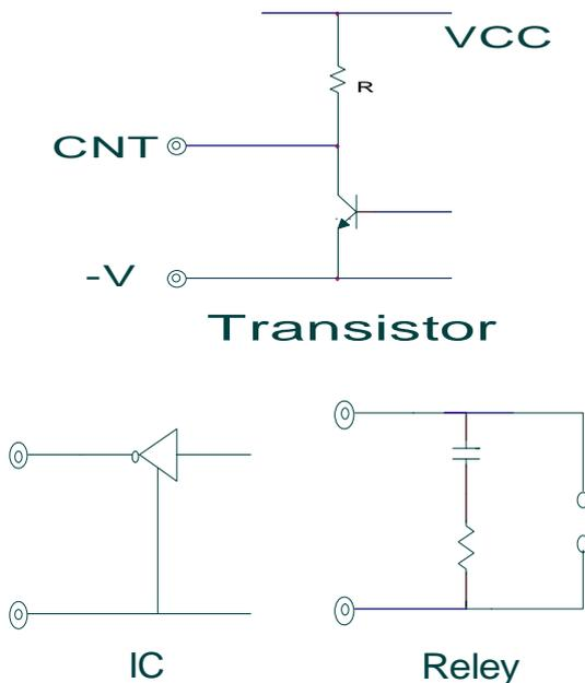
When CNT terminal is "LOW" level, fan out current is 1mA typ. When Vcc is applied, use 5V ~ Vcc 24V. When remote ON/OFF function is not used, please short between CNT and -V input.
